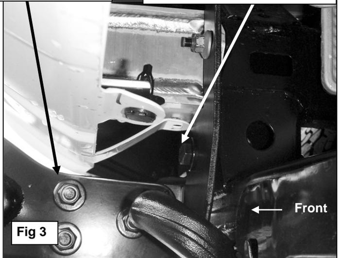
**NOTE:** It is not necessary but it may be easier to bolt the Top Brackets to the horizontal cross member in front of the radiator after the factory skid plate has been removed
