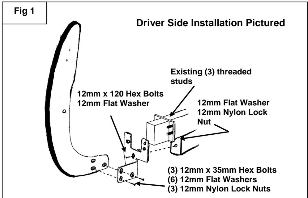
Factory hex nuts bolting driver side Frame Bracket to end of frame channel
